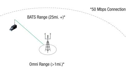
Directional microwave links, like those used in BATS-enabled systems, have proven ideal due to their longer range. Instead of saturating a small area with a wireless signal, these systems make use of signal power by directing the transmission to a specific recipient.
